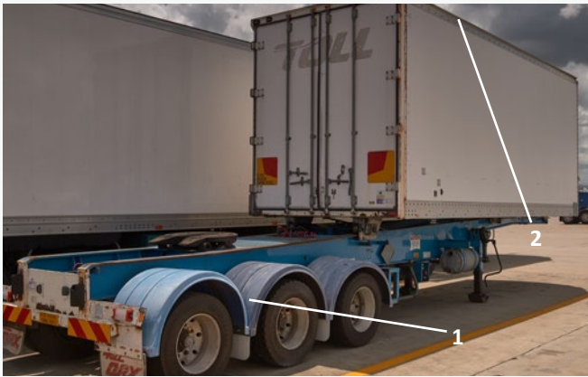
Figure 14.9 Secondary trailer structure components
