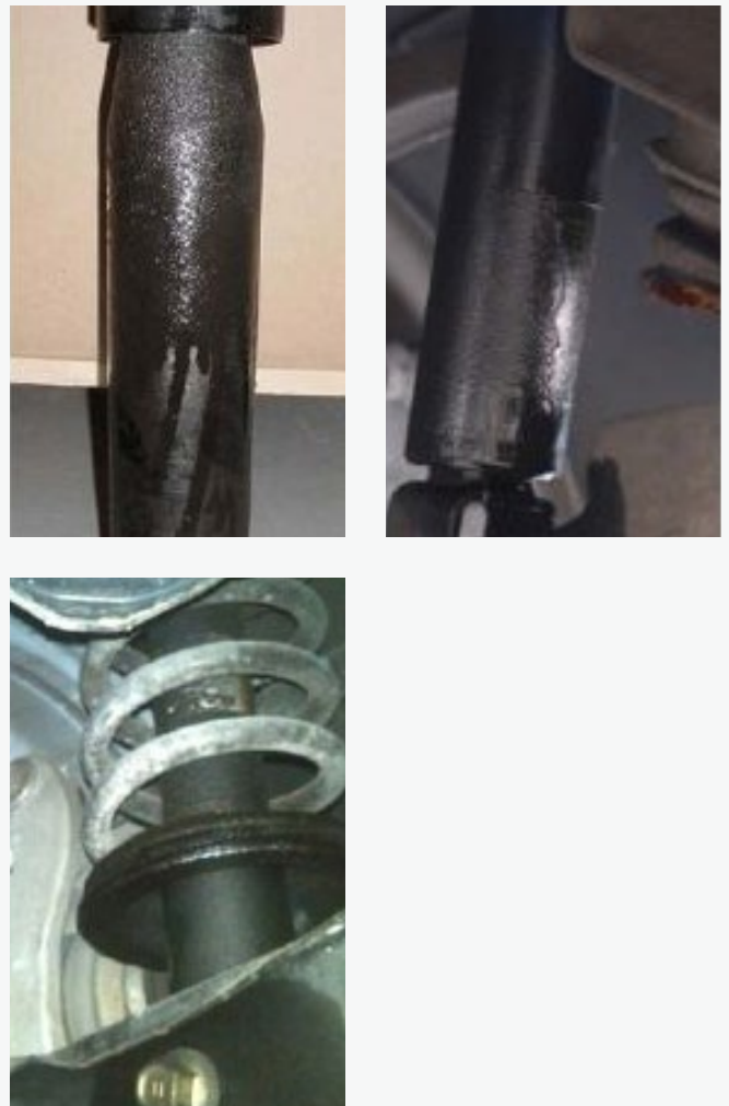
Figure 4.5 Examples of leaking shock absorbers
